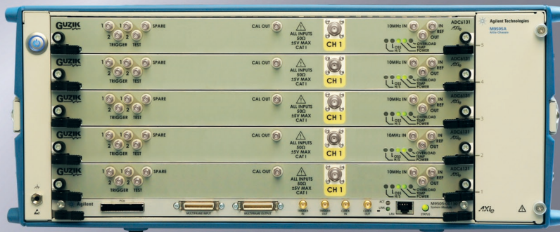
Five channels of 13 GHz BW with 40 GSa/s in the 4U 5 slot Keysight M9505A AXIe chassis
